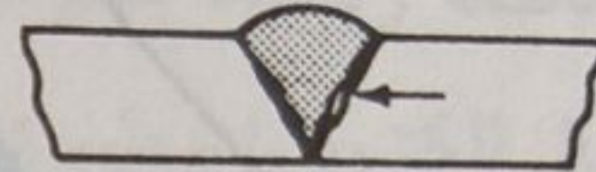
Lack of fusion
