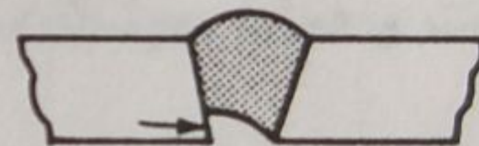
Excess root opening
